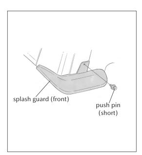
8. While pressing splash guard tight to panel install push pins (short).
