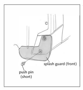
10. While pressing splash guard tight to panel install push pins (short).
