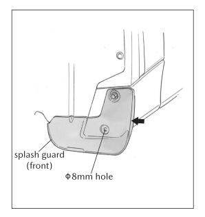
9. While pressing splash guard tight to panel drill hole in panel using part as a template, remove any burrs from hole.
