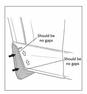
5. Press the splash guard (Front) against the vehicle so that there are no gaps between contact surfaces as shown.
