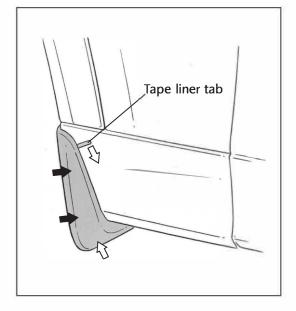
6. While pressing splash guard (Front) so there are no gaps remove tape using tab to pull down and out.
