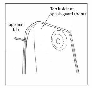
3. Fold tape liner tab facing out at top inside of splash guard (Front).
