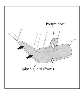
7. Using splash guard as a template drill  $\Phi 8$ mm hole in panel, remove any burrs from hole.
