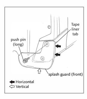
4. Set the splash guard (Front) against the vehicle with tape tab facing out, then install push pin (long).
