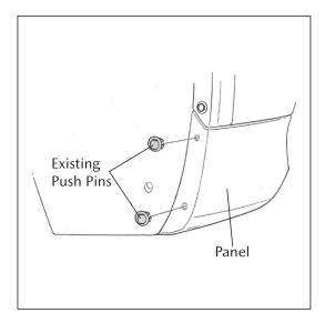
3. Remove existing push pins with slot screwdriver. (Discard)
