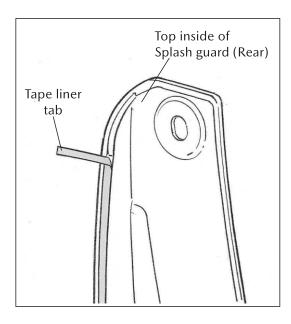
4. Fold tape liner tab facing out at top inside of splash guard (Rear).
