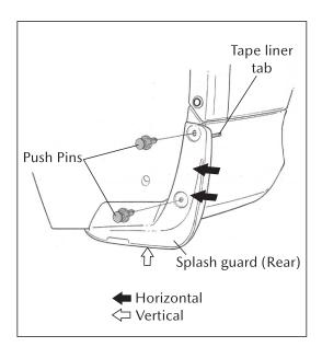
5. Set the splash guard (Rear) against the vehicle with tape tab facing out, then install push pins, while pressing splash guard tight to the panel.
