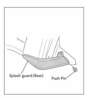
7. While pressing splash guard (Rear) tight to panel install push pin.
