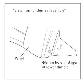
2. Use the drill to drill  $\Phi$ 8mm hole in stages as marked lower dimple, remove any burrs from hole.
