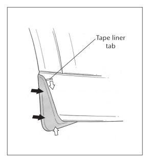
6. While pressing splash guard (Rear) so there are no gaps remove tape liner using tab to pull down and out.
