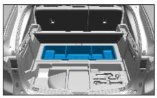
5. Insert cargo organizer into middle cargo sub-compartment, ensuring it is fully seated.
