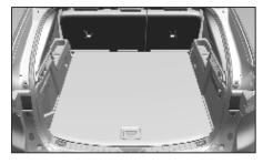
6. Unfold cargo floor board until flat and fully covering cargo sub-compartments.
