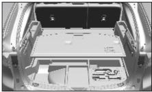
2. Fold rearward portion of cargo floor board upward.
